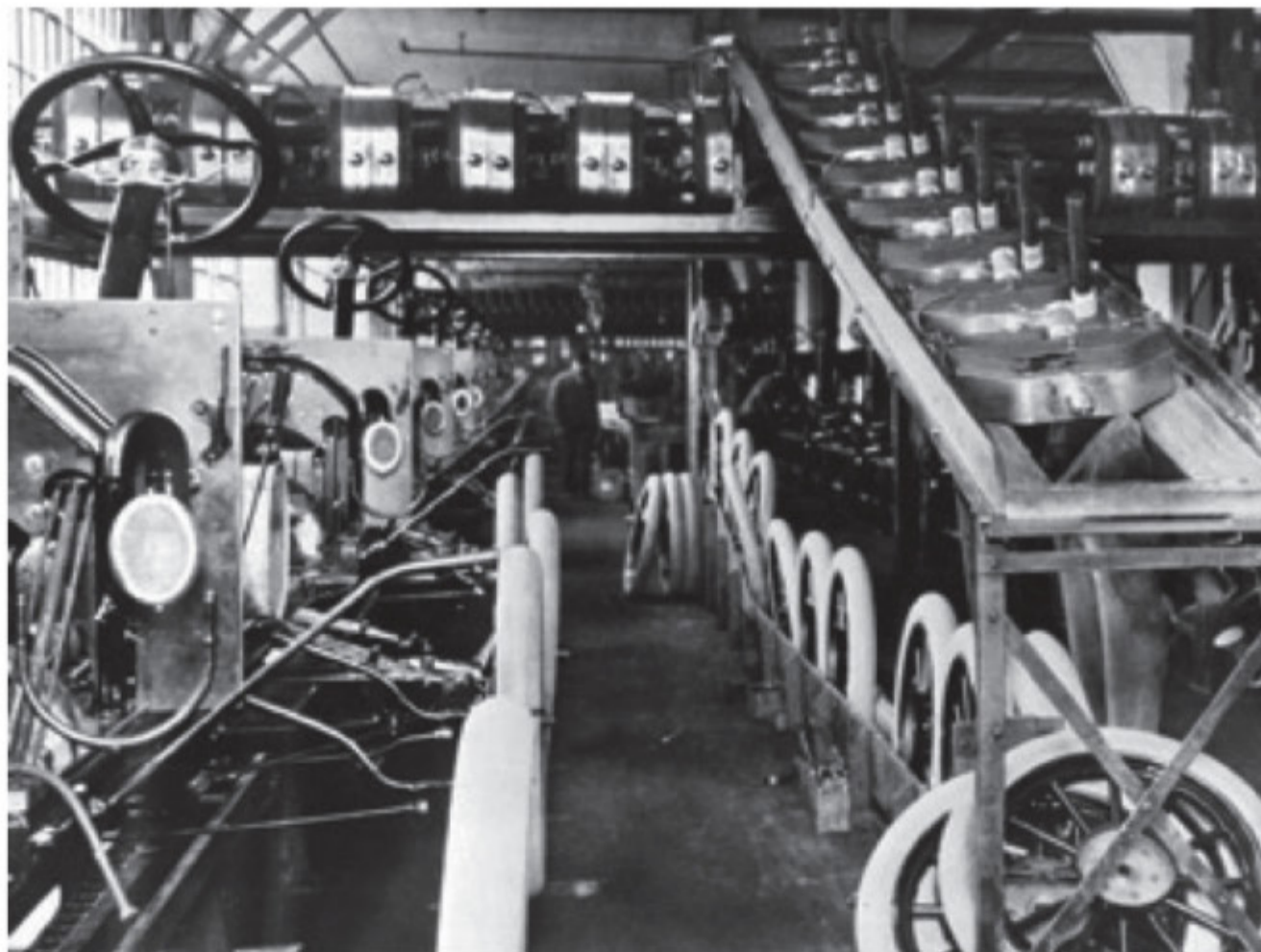
<The conveyor belt system first installed by Ford Motor Company in 1913>
